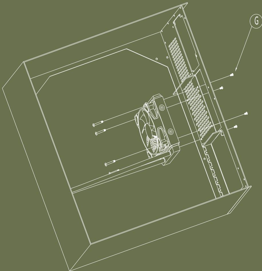
1. Instale as fans no radiador. (Pré-instalados)
